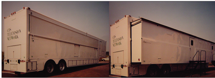
Figure 3.22 Equipment getting smaller didn't equate to more people space in trucks. It just meant more equipment could now be carried. As the number of sources increased, the amount of people required onboard during production also increased. To accommodate those folks, trucks that expanded out (expando) when parked arrived on the scene. (Source: A.F. Associates)
