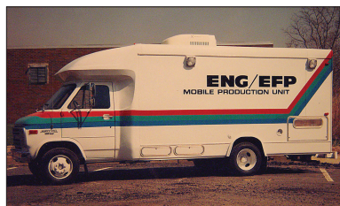
Figure 3.18 Conversely, trucks devoted to one- and two-camera productions got smaller. Trucks geared for single-camera operation became numerous, as a van could now carry the necessary camera, VTR and support equipment. Raw videotape footage could be captured in the field and edited back at the station. (Source: A.F. Associates)
