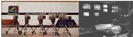
Figure 3.17 A 1970s vintage truck with Norelco PC-70s, the main competition for RCA's TK-44. In fact, the PC-70 became the prevalent truck camera of the time. Internally this trailer's production compartment was much more spacious than earlier trucks. Starting in the '70s, and accelerating through the '80s, equipment rapidly shrunk in size, allowing two things to happen. Trucks got bigger and smaller at the same time. The trucks geared for high-end productions got larger. Forty-foot trailers were common in the late 1970s; by the mid-80s 48-foot trucks were prevalent; and today, the maximum allowed FTC length of 53 feet is common.
