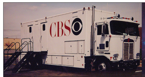
Figure 3.19 This D.C.-based CBS truck used for news shows in the late '70s and early '80s had up to six cameras and two VTRs, and could handle up to 12 more sources. (Source: A.F. Associates)
