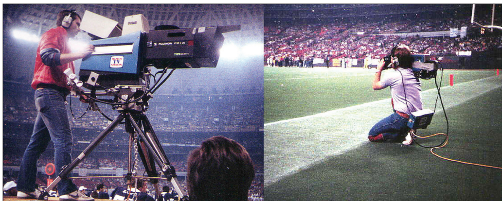
Figure 3.26 The triax camera had a major impact on remote operations. Instead of large cables from the truck to the camera, much thinner cables could be carried. This allowed for more cable, which meant more cameras, and more dispersed camera locations. Triax is a close cousin of the coax cable. Left is an RCA TK-47, right is an RCA TK-86.
