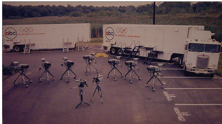
Figure 3.25 In the second half of the '70s, the handheld camera arrived on the scene. Thus, a mix of studio (also known as hard cameras) and handheld cameras became the complement of most trucks. Here another photo of Phase 7 shows its seven studio cameras, and two handheld (or soft) cameras on display. The handheld cameras are the front two cameras on tripods. (Source: A.F. Associates)
